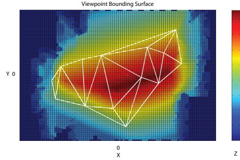
**Figure 1:** A  $100 \times 100$  grid of valid viewpoints color coded by  $z$ -value. A mesh connecting the original viewpoints in the input light field is shown in white. Note viewpoints in the central area are closer to the original sampled viewpoints; thus they can move much closer to the scene (larger  $z$ ) than peripheral viewpoints.
