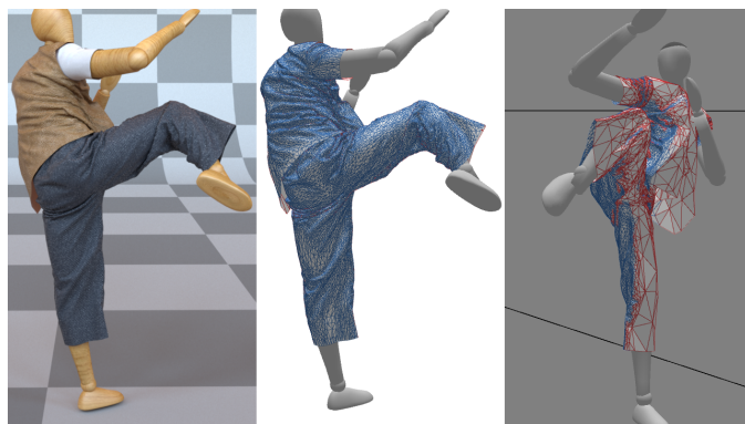
Fig. 1. The clothing on this character uses view-dependent simulation. Visible areas (blue) are simulated at high resolution, as measured in screen-space. Areas not visible to the camera (red) are simulated at reduced resolution. The first two images show views from the camera's perspective. The rightmost image shows an outside perspective with the camera's view frustum drawn in black wireframe.
