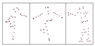
Figure 2. These images show marker configurations typical of the data from an optical motion capture system. Each image corresponds to one frame for one of our human subjects.
