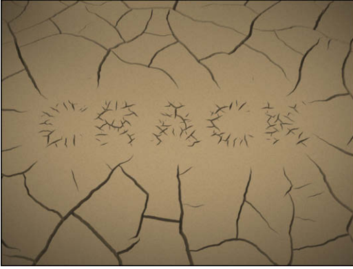
Fig. 9. We can use an input image, such as the letters “crack”, to define areas with high stress and produce the small scale cracks shown in the center. We then created the large scale cracks with a second simulation by decreasing the stress in the letter region and reinitializing the surrounding area to uniform shrinkage.
