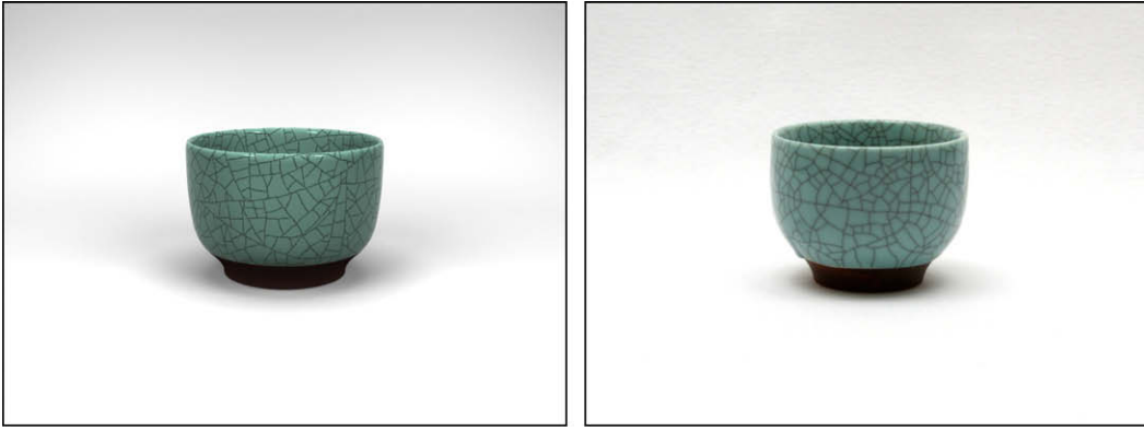
Fig. 5. A rendered example of a crackle glaze cup (left) compared to a photograph (right). Our algorithm generates this effect by initializing the stress field to uniform shrinkage over the surface and evolving it with uniform tension. Total computation time was 31 min with a 39,611 triangle input mesh.
