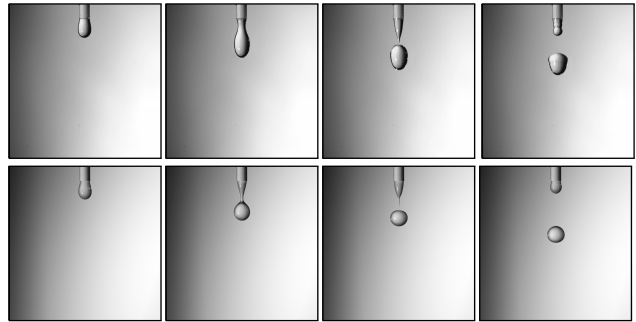
Fig. 11: Frames from a droplet pinch-off. We compare real video (top) with a simulated flow velocity of 0.11 mm/s (bottom).
