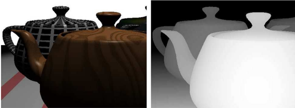
Fig. 12. Original teapot scene (left) and its associated depth information (right). © 2005 by B.A. Barsky.
