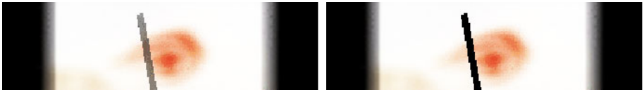
Fig. 4. A focused black line occludes a defocused book. Left: The standard linear filtering method results in a translucent occluding object, which is incorrect in this scene. Right: The occlusion problem is solved using the RDB, and the black line is properly opaque. (Courtesy of Mikio Shinya [18].)
