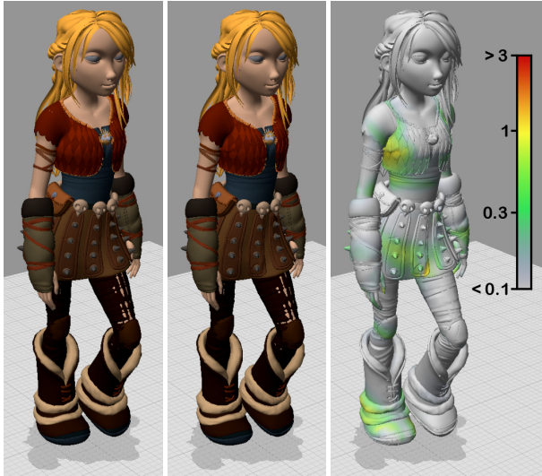
Fig. 4. Side-by-side comparison of the ground truth mesh (left) and the approximation (center). The vertices of the approximated mesh are colored to indicate the per-vertex distance error (right). Errors above and below the range of the scale are clamped to the ends of the color range. All distances are measured in centimeters.
