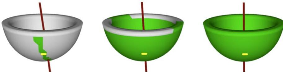
Our fitting algorithm starts from a user stroke on the model (shown in yellow). We then iteratively fit a sweep model to those points, and region grow to expand the selection to those surface points that also fit within some given error tolerance. The problem of fitting a field to any given selection is solved by a small (7x7) generalized eigenvalue problem, and the whole process tends to converge in only 2-3 iterations, making it very fast in practice.
