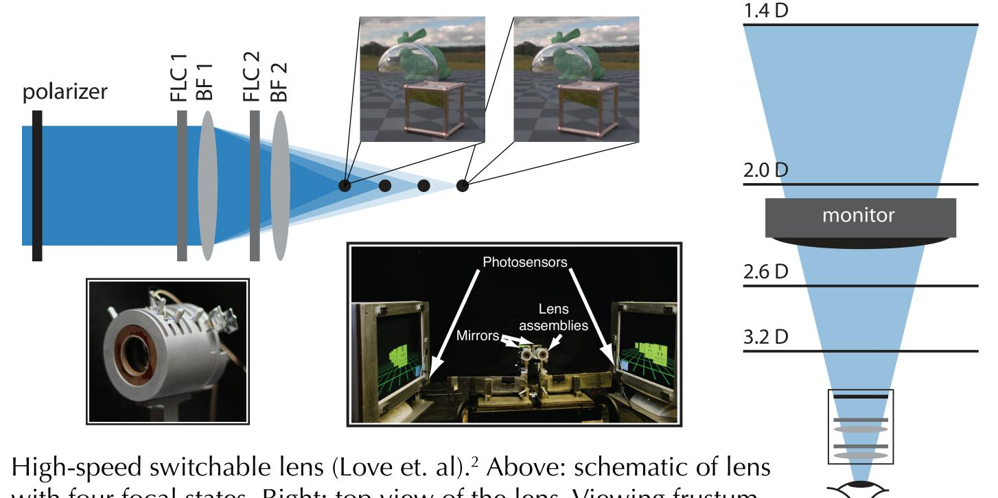
with four focal states. Right: top view of the lens. Viewing frustum in blue, horizontal lines show focal distances of four lens states.
